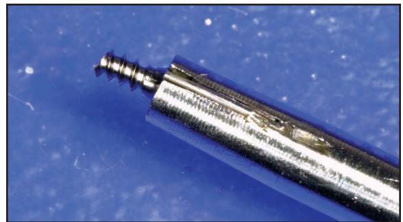
**Fig. 6 Screw broken during insertion.**
